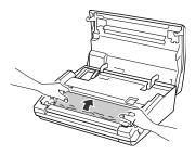
5. Replace the roller. Make sure the roller's tabs lock in place.
